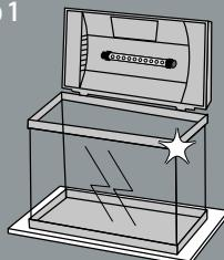
Place aquarium on a smooth, horizontal surface with an adequate load-bearing capacity. Do not place the aquarium on electrical appliances or on furniture with surfaces which are liable to staining by water.
